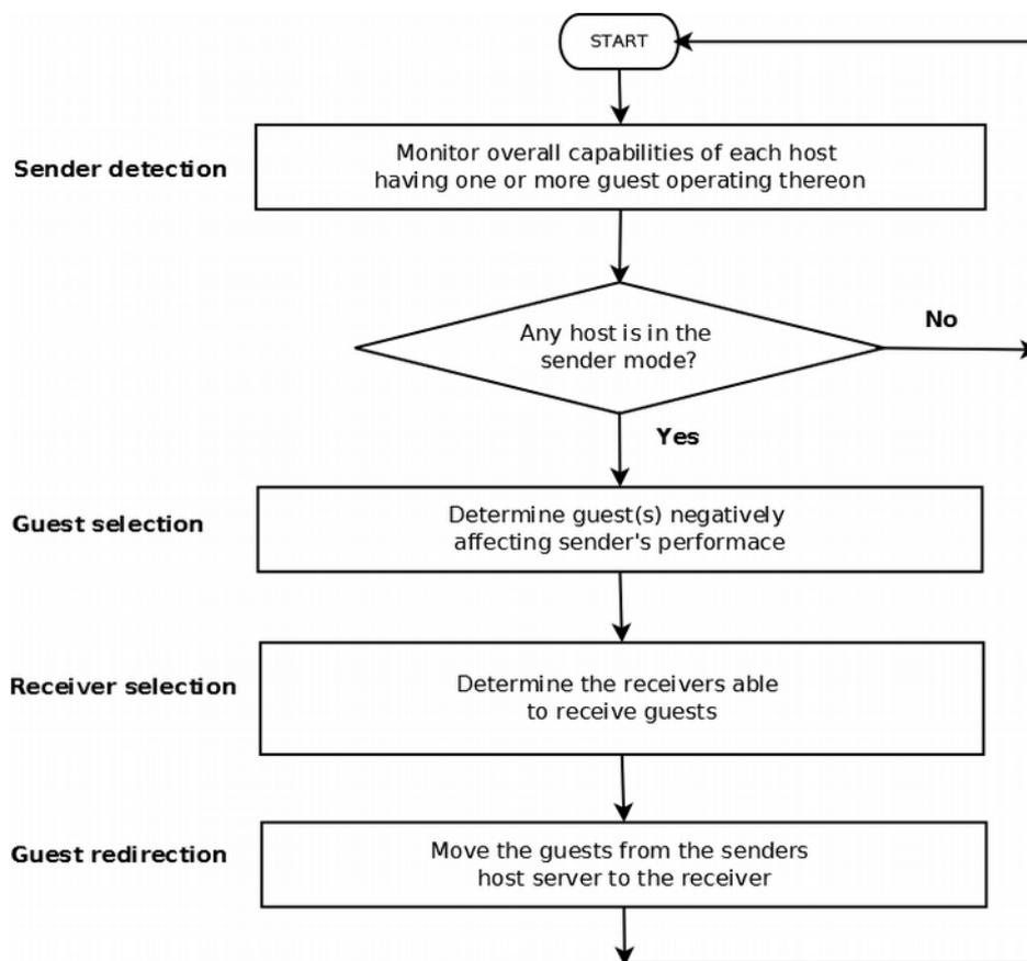
Figure 1: Flow diagram of the virtual machine migration process.
