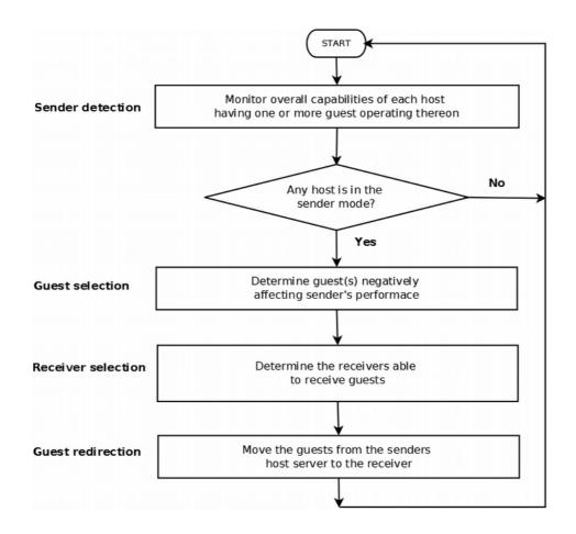
Figure 1: Flow diagram of the virtual machine migration process.
