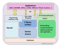
Figure 3. Software schema
