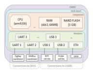
Figure 2. Hardware schema
